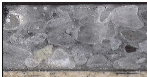
*Section of a 3 mm layer of NM Solid 515*
